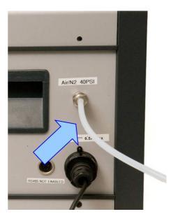
Remove the nylon cap from the Air Inlet port on the rear of the system.
