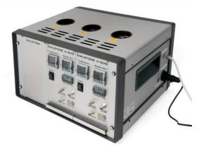
V-OVG is designed to generate chemical vapours. To limit the user's exposure to these vapours it is strongly recommended that the V-OVG be operated in a fume hood, or well-ventilated space.
