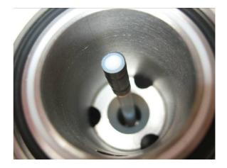
To insert a permeation source into the oven, first disconnect the air supply to the V-OVG and wait for the unit to depressurise. (Sample and Exhaust Flows should read 0 ml min<sup>-1</sup>). Unscrew the black lid of the oven, located on the top surface of the V-OVG.
