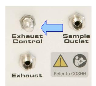
Remove the nylon cap from the Exhaust port on the front of each V-OVG sub-unit supplied with the system.
