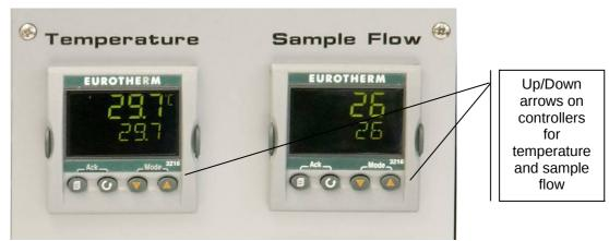
Using the Up-Down arrows on the temperature controller set your intended incubation temperature. Before loading your first permeation source it is sensible to wait for the oven temperature to stabilize at the set-point.
