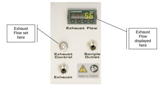
To prevent a potentially dangerous build up of vapour in the permeation oven it is essential that a small Exhaust Flow is set before incubating your first permeation source.
