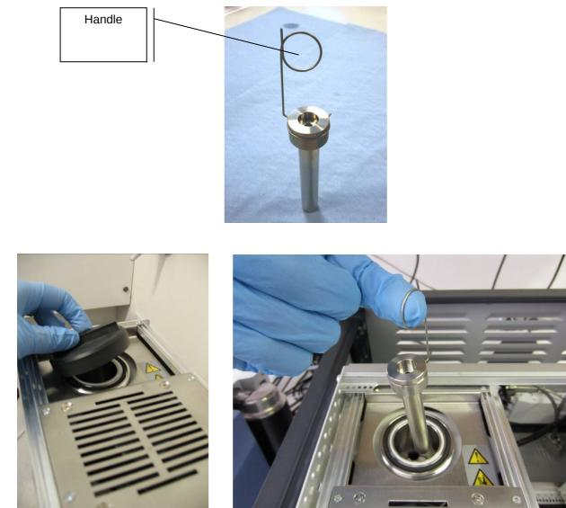
To insert a wafer device into the oven, first disconnect the air supply to the V-OVG and wait for the unit to depressurise. (Sample and Exhaust Flows should read 0 ml min<sup>-1</sup>). Unscrew the black lid of the oven, located on the top surface of the V-OVG.
