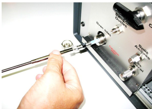
Figure 9 – Always use the supplied extraction tool
